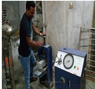
Figure 6: Experimental Setup for Flexural Strength
